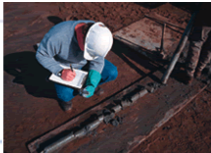
An employee of an energy company records a core sampling test of the soil.
