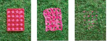
These photos show the breakdown of a newly developed plastic during a one-hour period. Created by Australian scientists, the plastic is made of cornstarch and disintegrates rapidly when exposed to water. This technology could help eliminate the 24 million tons of plastic that end up in American landfills every year.
